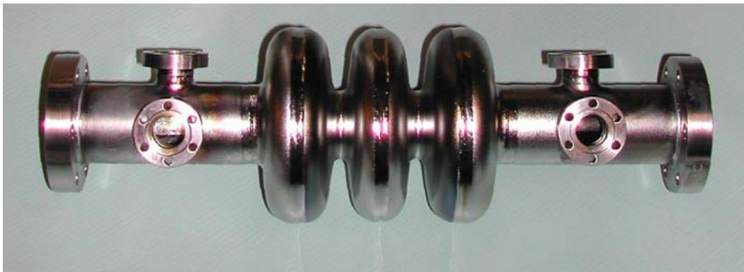
FIGURE 2.7-9. Photo of a 3.9GHz 3-cell deflecting cavity built at Fermilab, which achieved 7.5MV/m.
