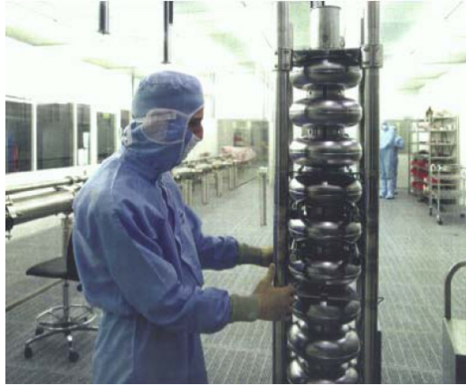
FIGURE 3.6-2. A TTF cavity assembled and prepared for RF qualification testing.
