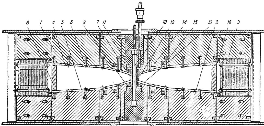
Fig. 3. Schematic cross-section of the first variant of the assembly B-3. 1, 2 - magnet poles; 3 - locking yoke; 4, 5 - vacuum chamber covers; 6 - vacuum cover bolts; 7 - internal shell; 8 - external shell; 9, 13 - shielding system; 10 - core; 11 - core winding; 12 - injector; 14, 15 - "slot" windings; 16 - chief field winding.
