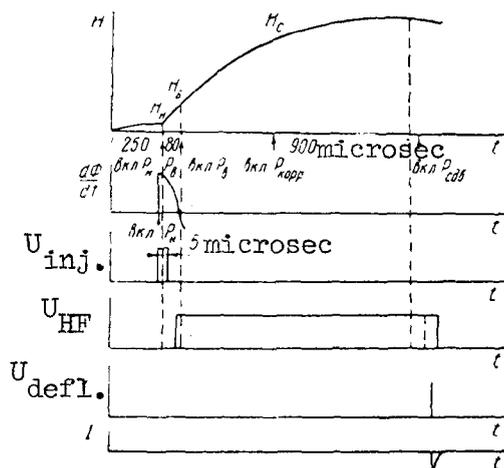
Fig. 2. Scheme of process sequence in the acceleration cycle of the assembly B-2C.
