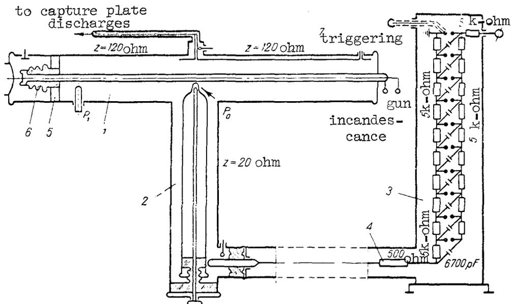
Fig. 6. Injector diagram.
