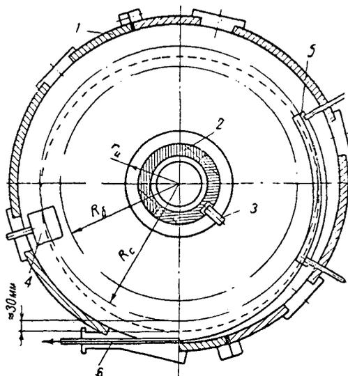
Fig. 1. Simplified cross-section of the acceleration chamber of the synchrotron B-2C. 1 - external shell; 2 - internal shell; 3 - injector "gun"; 4 - resonator; 5 - deflector; 6 - extraction channel;  $r_i$  - injection radius;  $R_\beta$  - position of the betatron orbit;  $R_c$  - position of the synchrotron orbit; - - - extraction trajectory.
