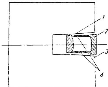
Fig. 7. Cross-section of the synchrotron B-3M electromagnet. 1 - internal bus of the electromagnet; 2 - external bus of the electromagnet; 3 - magnetic circuit; 4 - vacuum covers.
