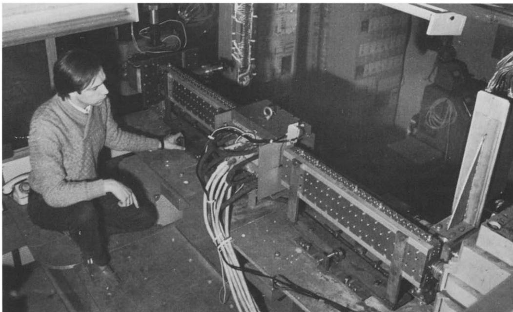
Fig. 13. The OK-3 magnetic system installed on VEPP-3.
