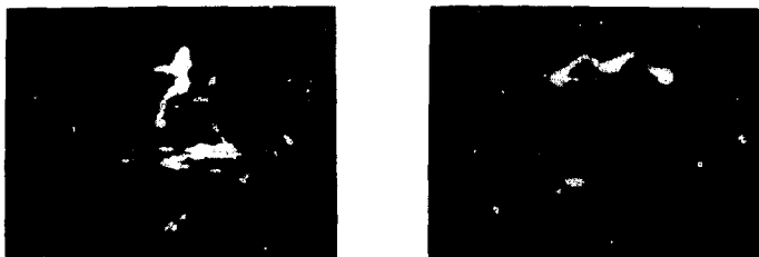
Figure 15. Cosmic rays tracks recorded with the imaging chamber.
