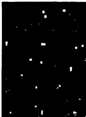
Fig. 10. Visual output from a CCD matrix irradiated with particles. The size of the presented part is 1 \times 1 \text{ cm}^2 [3].
