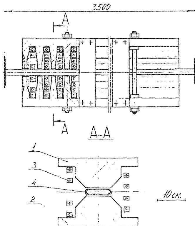
FIG. 1. Cross section of the undulator.
