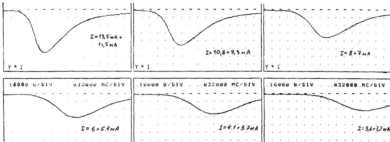
FIG. 7. Time dependence of outgoing radiation power of the OK under different values of electron bunch current.
