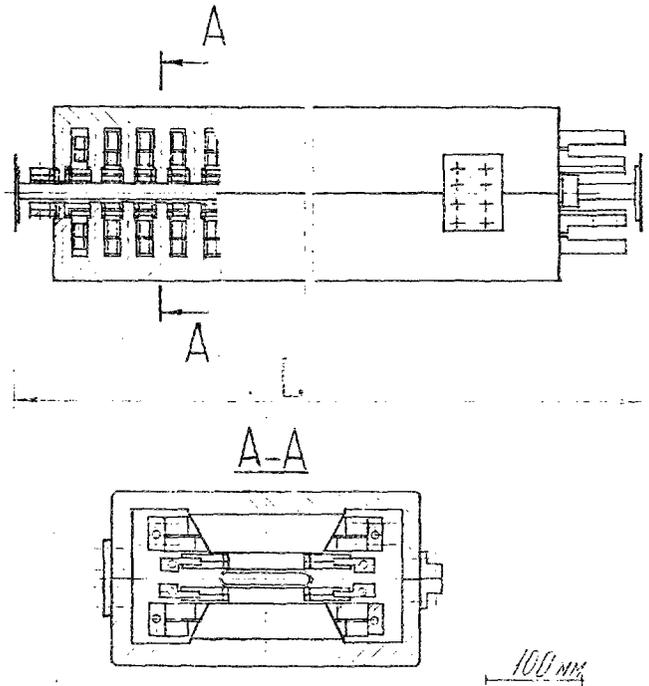
FIG. 2. Cross section of the undulator under construction.
