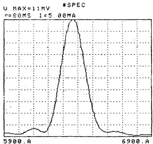
FIG. 3. Spontaneous radiation spectrum from one undulator.
