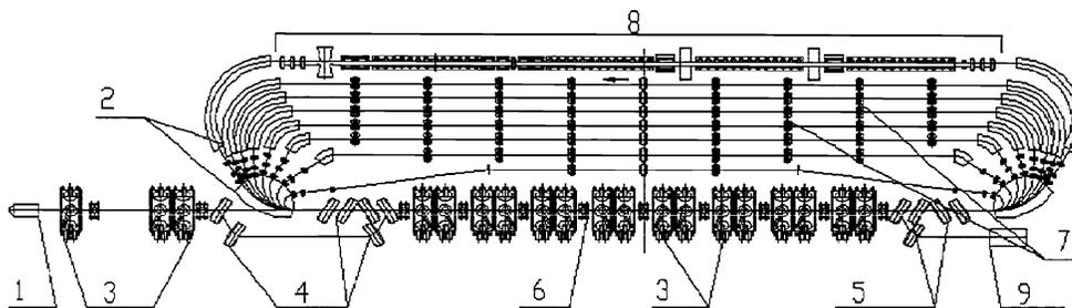
Fig. 1. The accelerator-recuperator layout. 1 - 300 keV electron gun; 2 - bending magnets; 3 - RF resonators; 4, 5 - injection and extraction magnets; 6 - focusing solenoids; 7 - straight sections with quadrupoles; 8 - the FEL magnetic system; 9 - the beam dump.
