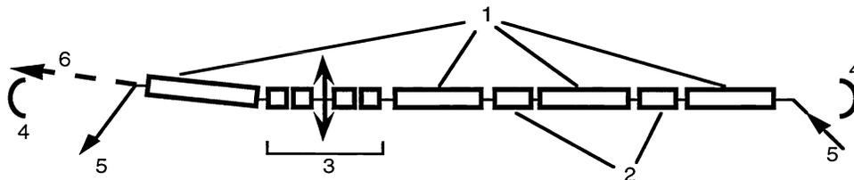
Fig. 2. The layout of the FEL magnetic system. 1 - undulators; 2 - dispersive sections; 3 - achromatic bend; 4 - mirrors; 5 - electron beam; 6 - output coherent radiation.
