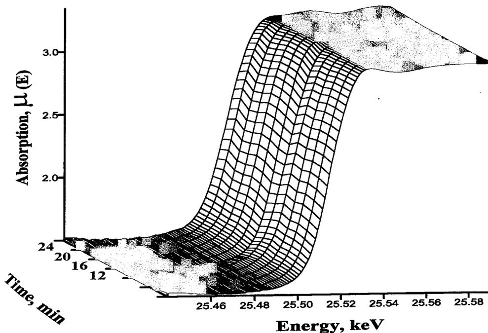
Figure 2: Evolution of the x-ray fine structure near Ag-K edge for the reaction :  $\text{AgSt} + \text{Red} \rightarrow \text{Ag} + \text{HSt}$  at  $T=80^\circ\text{C}$ .
