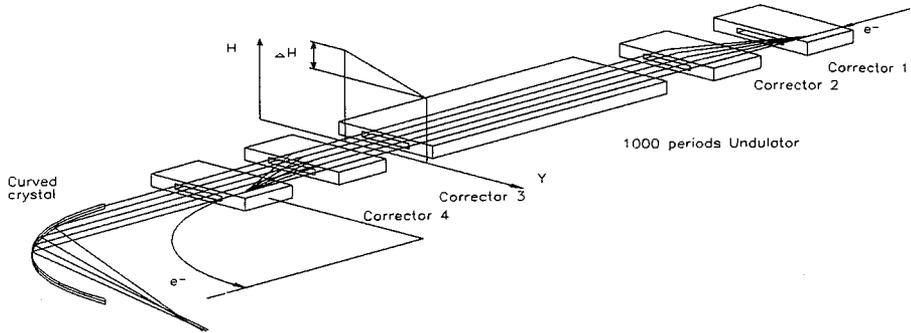
**Figure 3:** The proposed scheme for the XANES registration by electron beam position scanning at 1000 pole undulator with variable field, the gradient of which is perpendicular to the trajectory of the electrons. SR beams of different energy correspond to each electron orbit.
