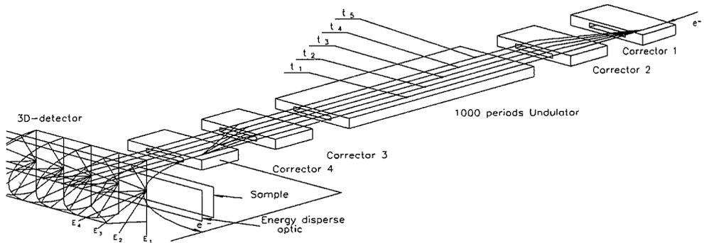
**Figure 4:** The proposed scheme for the XANES registration by electron beam position scanning at 1000 pole undulator with a variable phase shift. Each electron orbit corresponds to the SR beam which, in turn, corresponds to different time. A SR beam from each bunch diffracts from energy-dispersive elements, passes through a sample and then is registered by its own linear detector (one detector for each bunch). Thus, the magnetic field scan in the correctors is the scan in time.
