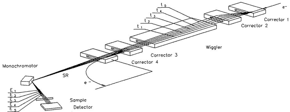
**Figure 1:** XANES registration by electron beam position scanning at VEPP-3. Originally the monochromator is set up so that it receives the photons from undistorted orbit  $t_1$ . Then the orbit is distorted to the maximum deformed orbit  $t_5$  and the scanning procedure begins involving slow changes of the orbit from  $t_5$  to  $t_1$ . For each electron orbit,  $t_1$ - $t_5$  corresponds to the SR beam with the energy  $E_1$ - $E_5$ .
