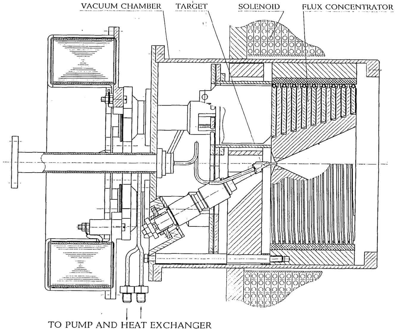
Fig. 19- Flux concentrator for positron collection with liquid lead target of the coaxial type.
