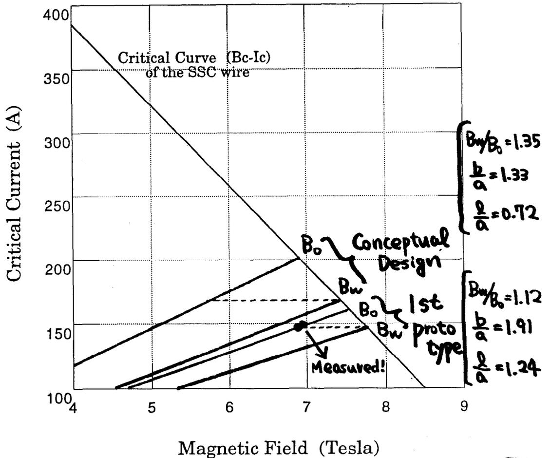
Achieved the performance which is close to the limit of wire material with 1st prototype !
