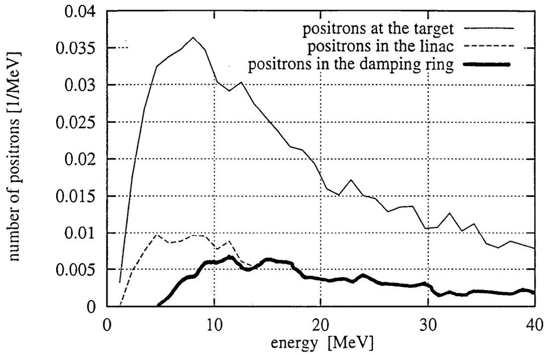
Energy distribution of the positrons emerging from the target (solid line) and the fraction of captured positrons (dashed lines).
