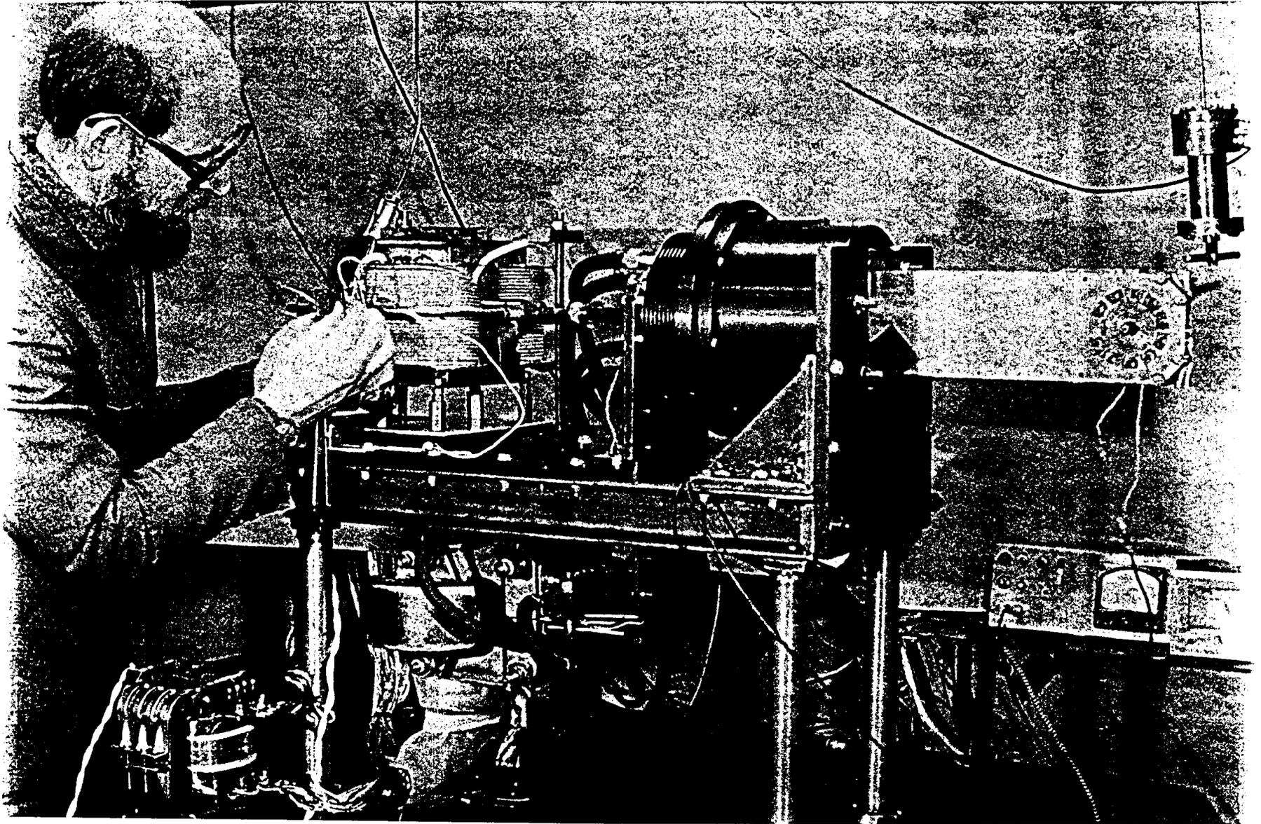
Fig. 16- Photo of a liquid lithium lens device with pump, matching transformer, and heaters.
