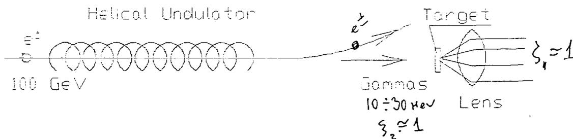
**The helical undulator converter insertion**
