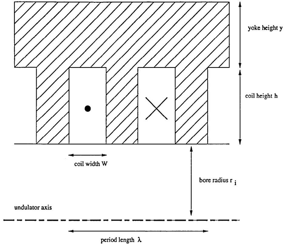
**Cross-section of an undulator with iron between the conductors and return yoke (shaded area).**
