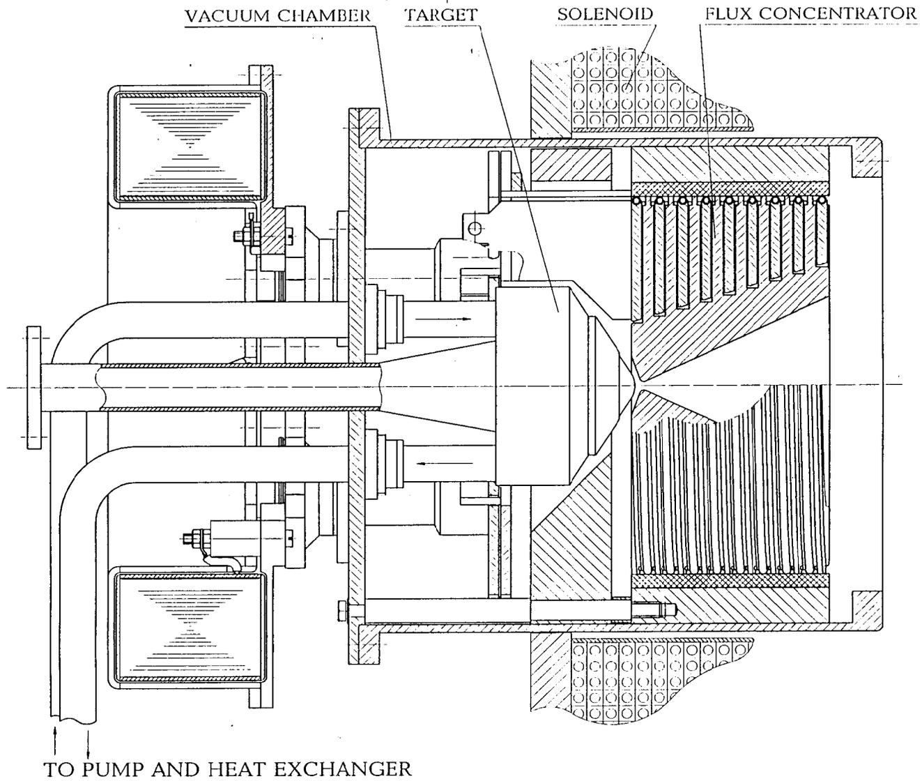
Fig. 23- Flux concentrator with liquid lead jet target.
