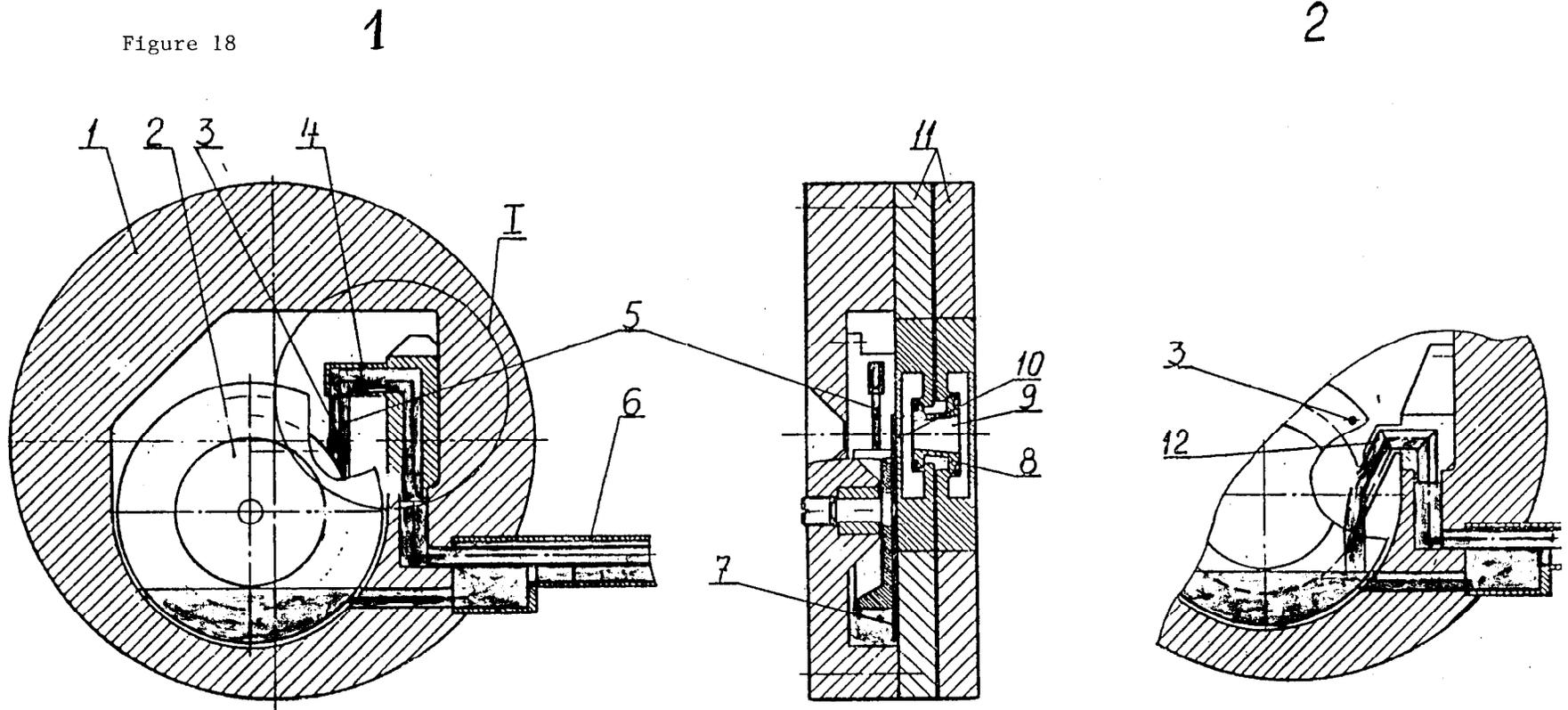
Target of the VLEPP conversion system: variant 1: mercury jet; variant 2: tungsten disk;
