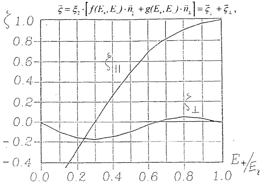
The longitudinal polarization of the positron created as a function of its fractional energy
