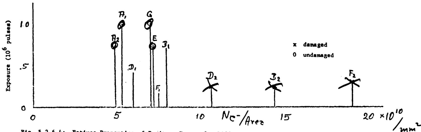
Fig. 5.2.6.4: Fatigue Properties of Positron Target for Different Electron Beam Densities
