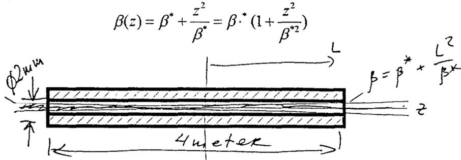
Beam size at the out of the undulator changes only 10%  $\rightarrow \frac{L^2}{\beta^{*2}} \approx 0.2$
