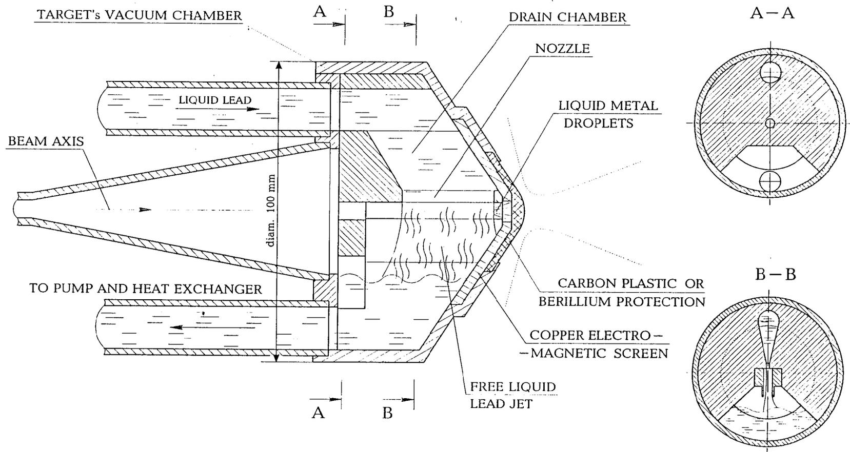
Conversion Liquid Lead Target
