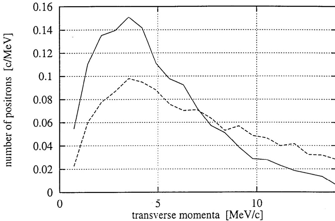
Comparison of transverse momenta for a SLC like source ( $6X_0$ , W, dotted line) and a thin target driven by wiggler photons ( $0.4 X_0$ , Ti, solid line).
