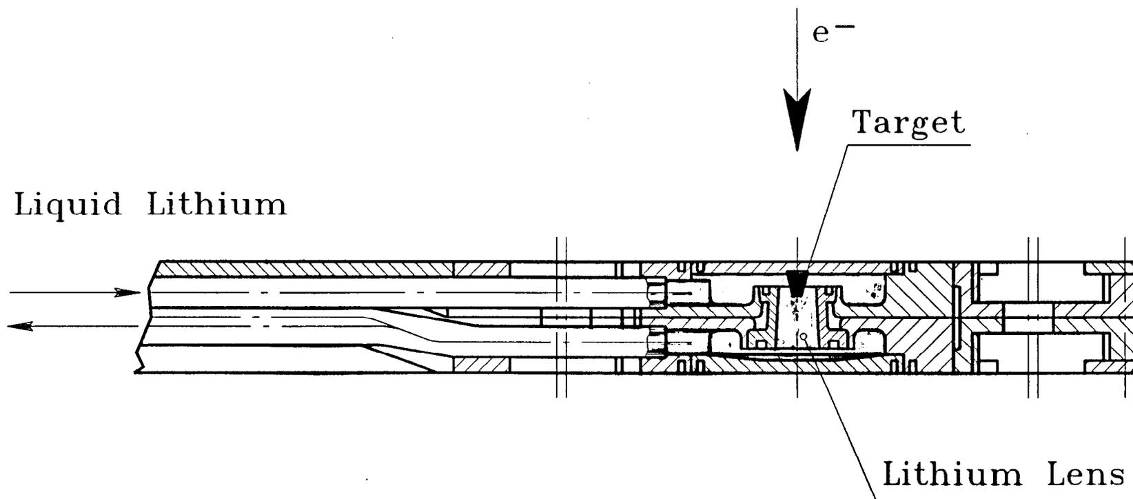
Fig. 13- The liquid lithium lens for the quarter-wave transformation of positron beam emittance. The lens length is 1 cm, field gradient  $G= 20$  T/cm, repetition rate 150 Hz. The tungsten target is cooled by flowing liquid lithium.
