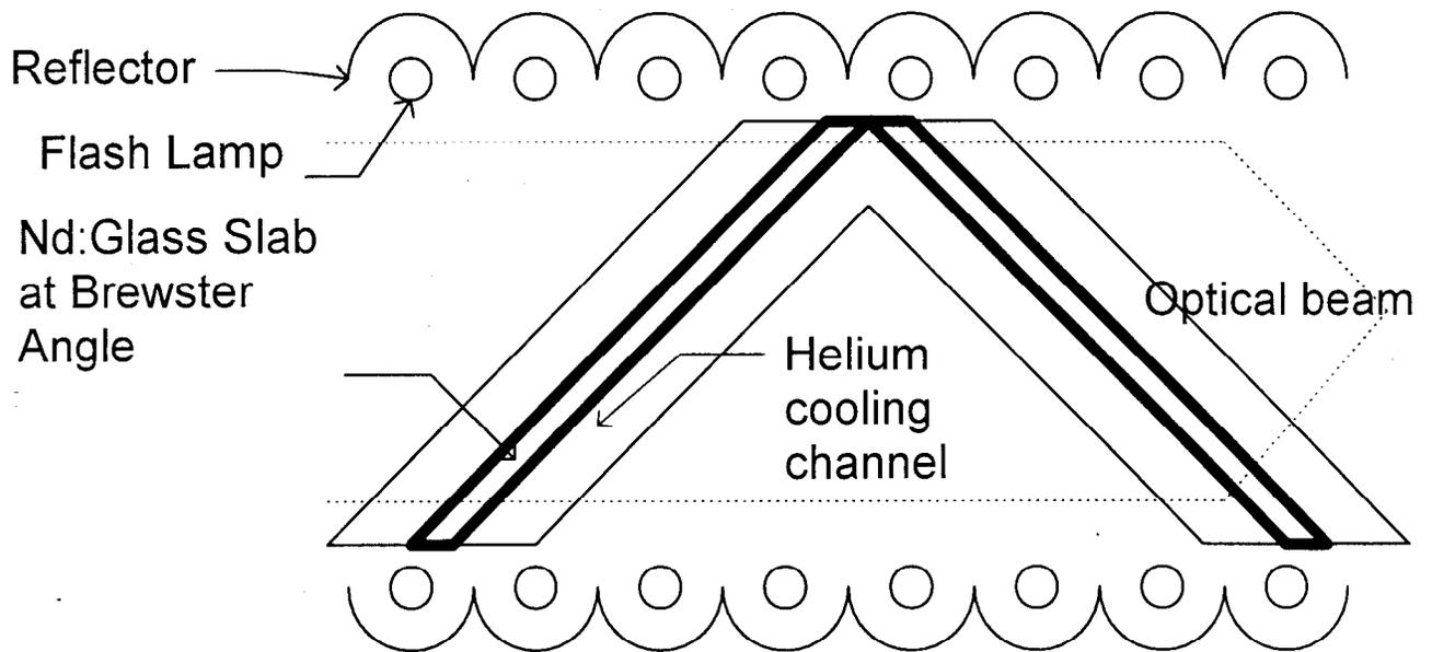
We can calculate the required mode area from the required macropulse energy (50J) and the saturation fluence (5.4J/cm<sup>2</sup>) to get an approximate mode area of 10cm<sup>2</sup>. Allowing for mode clearance, this is probably a 6cm X 12cm plate.
