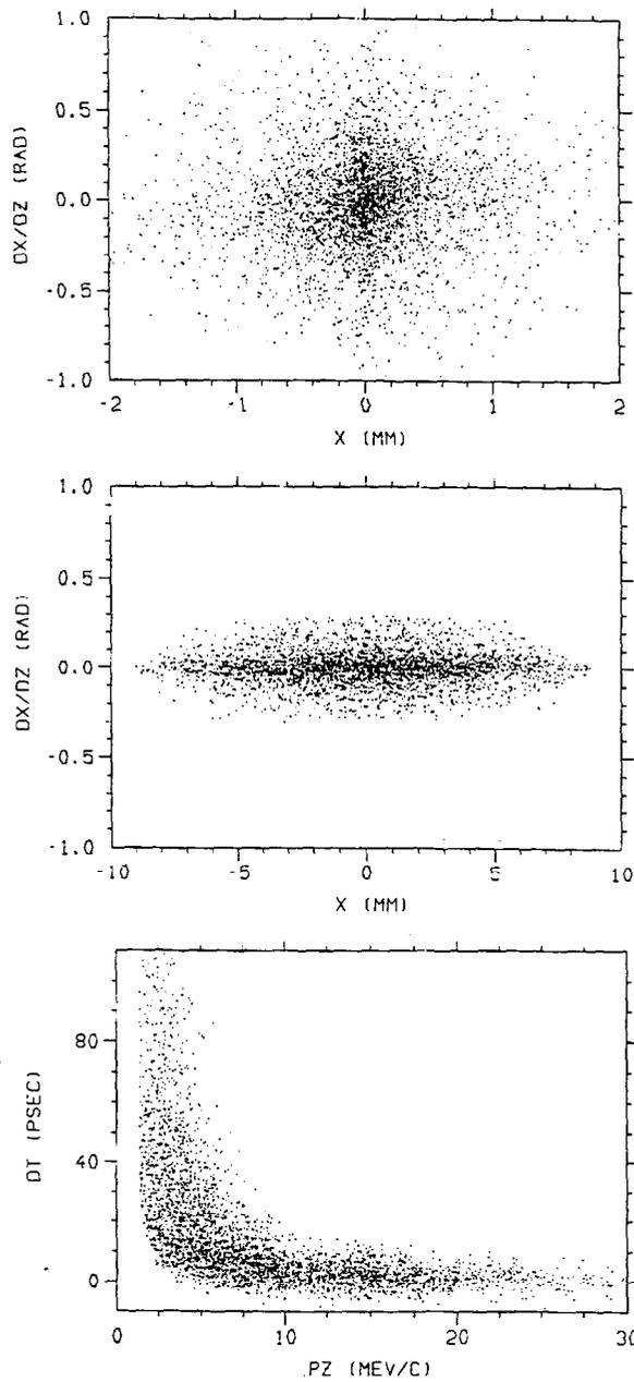
Figure 4. Phase space transformations. (a) EGS simulated phase space at target exit; (b) Transverse phase space at exit of FC ( $z = 140$  mm) as simulated by ETRANS; (c) Longitudinal phase space at exit of FC, also ETRANS.
