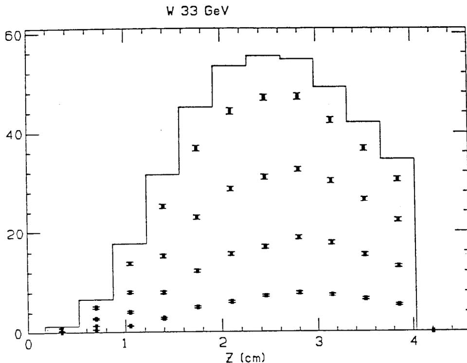
Fig. 2. Positron flux in tungsten per incident electron vs  $z$  for incident energy of 33 GeV. The different curves are for successively bigger cutoffs in maximum positron energy of 5, 10, 20, 50, and 100 MeV. The minimum energy cutoff is 2 MeV. The  $z$  bins are one radiation length. Note the shower maximum is around seven radiation lengths for this energy. The calculation covers the first eleven radiation lengths.
