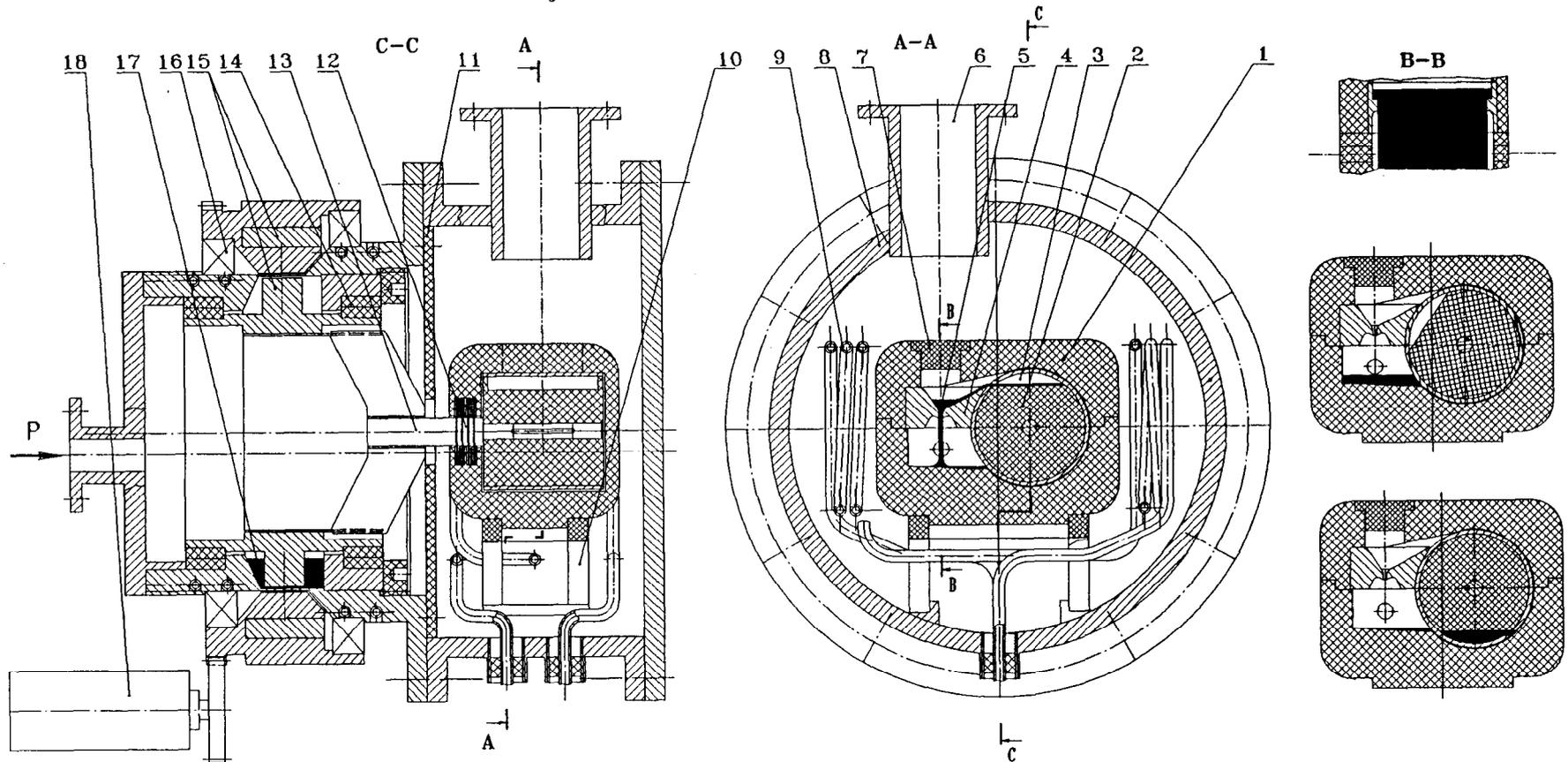
1-graphite body of pump; 2-graphite revolving cylinder with molibdenum envelope; 3-rilling cavity; 4-molibdenum drain chamber; 5-liquid metal jet and beam axis; 6-observation window; 7-closing insert; 8-vacuum chamber body; 9-RF heater; 10-ceramic support; 11-heat screen; 12-separating labyrinth; 13-revolving axle; 14-graphite bearing; 15-magnetic muff; 16-bearing; 17-gallium-indium cooler; 18-driver motor.
