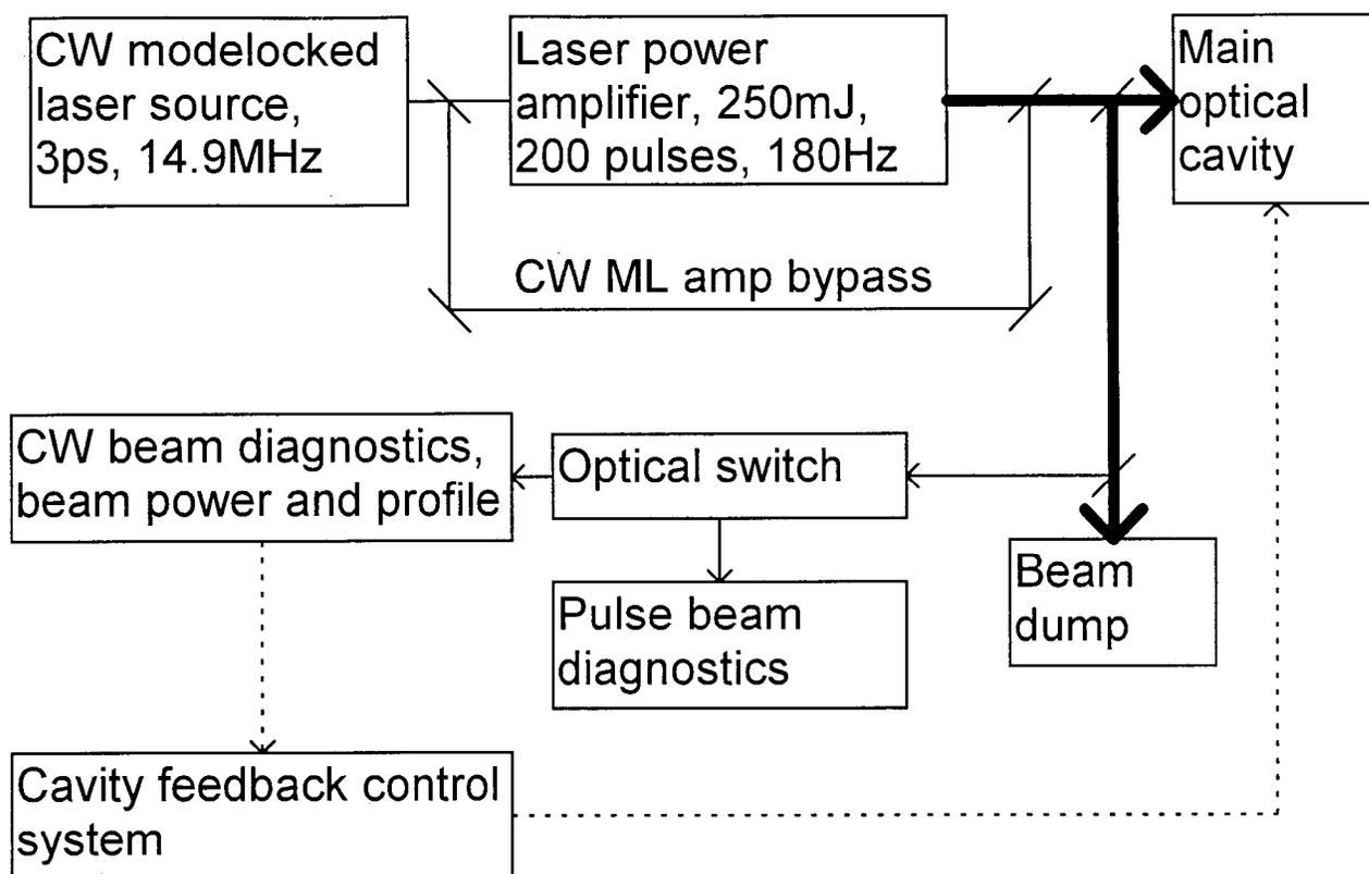
The cavity mirrors will be located in the accelerator vacuum system (transmitting optics is not possible at the intra-cavity power levels), so they should be immune to most external effects. Interferometric gravity wave detectors have used optical cavities with mirrors stabilized against external (eg seismic) effects many orders of magnitude better than our requirements.
