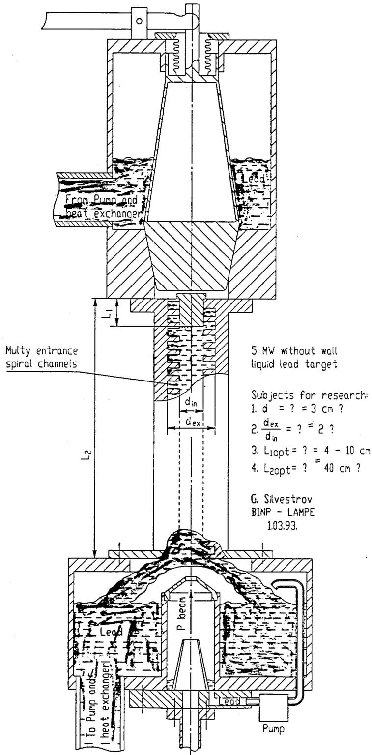
Fig. 12- Conceptual design of the Mega-Watt centrifugal-type liquid-lead target for the Neutron Spallation Source.
