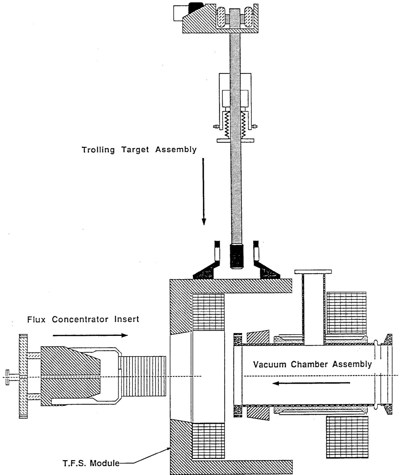
**Target/Flux Concentrator/Tapered Field Solenoid
