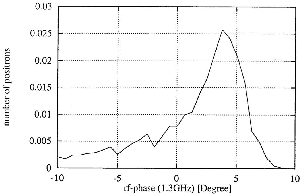
Longitudinal beam profile of the positrons behind the matching device. Only the fraction of positrons within  $\pm 7.5^\circ$  is accepted in the simulations.
