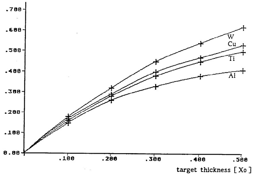
Fig. 1.11 Positron yield for various materials obtained with wiggler photons ( $B=1.7$  T,  $S=1$  m) versus target thickness in units of radiation length;  $E=250$  GeV
