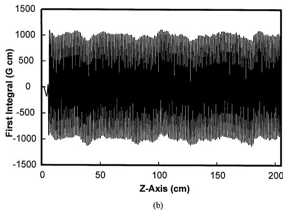
Fig. 4. (a) Measured magnetic field trace of the constructed undulator and (b) the first integral of the field.
