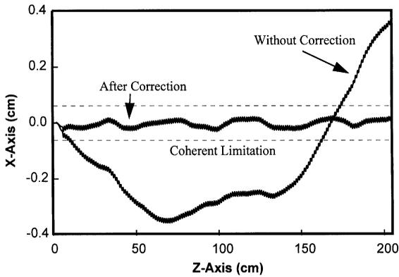
Fig. 5. Calculated electron trajectory obtained from the results of magnetic measurement without correction and with the help of eight correction coils.
