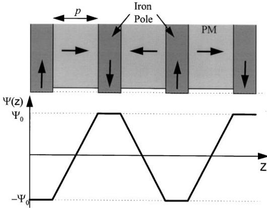
Fig. 2. Distribution of the scalar magnetic potential along the  $z$  axis through the end surface of the iron pole.
