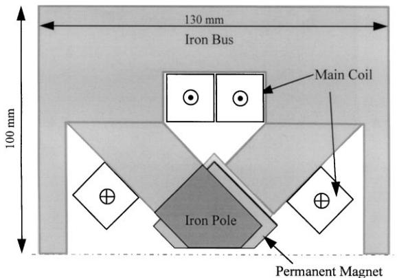
Fig. 1. Upper part drawing of the equipotential-bus EM undulator.
