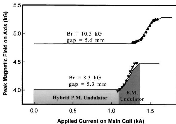
Fig. 3. Calculated (line) and measured (solid circle and triangle) peak magnetic field on axis as a function of applied current on the main coil.
