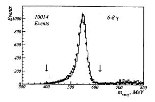
The recoil mass of the most energetic photon in an event. Points – data, histogram – simulation
