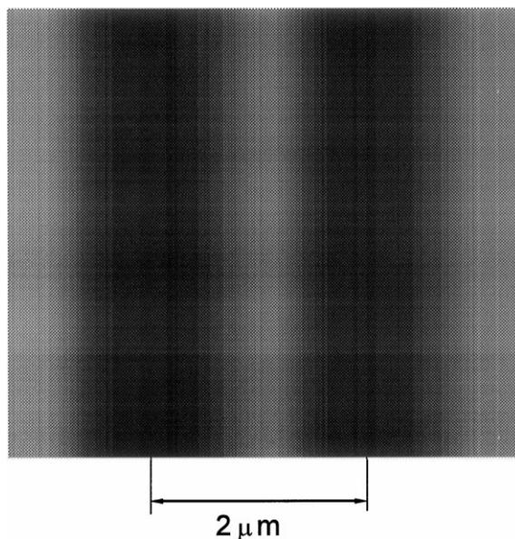
Fig. 1. Examples of image: 2  $\mu\text{m}$  test-structure (gold). The luminescence was read out by point-to-point scanning and registration in the photon account mode.
