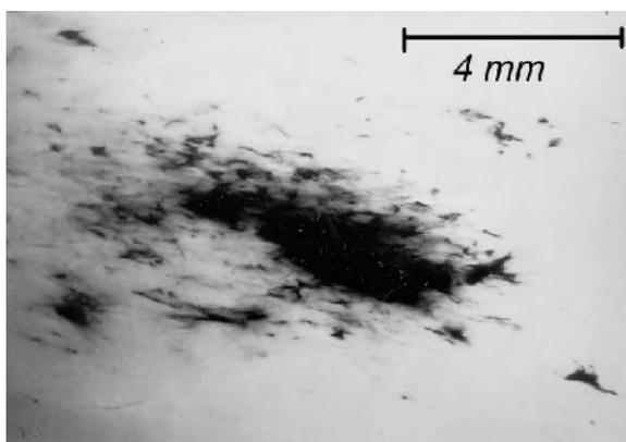
Fig. 7. Wide spots of the very imperfect sample SK-36 consist of a lot of reflexes of intricate form and size.
