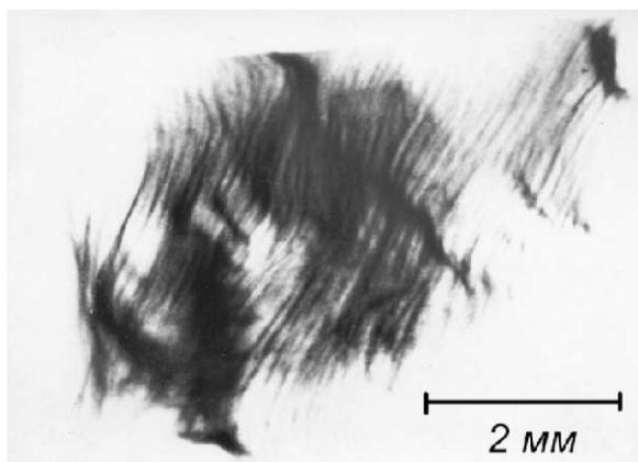
Fig. 2. A slip system's deformation bands throughout the crystal (sample BP-1/97).
