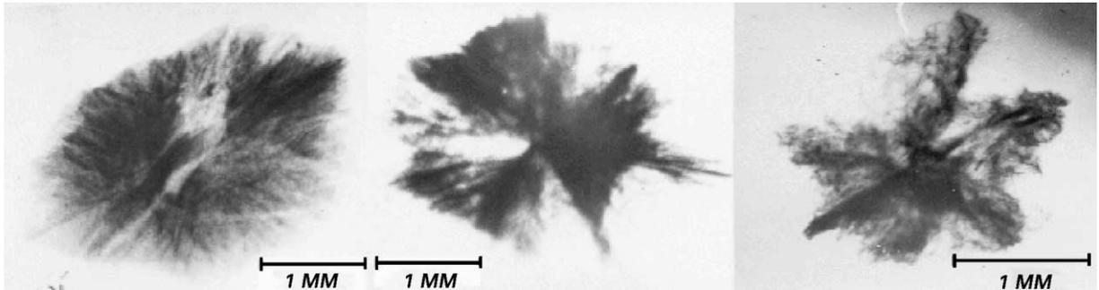
Fig. 8. A row of topograms of diamond cuboids to illustrate the fine-fibre (left, sample Z-1), coarse-fibre (centre, sample Z-2) and dendrite-like (right, sample Z-9) structure.
