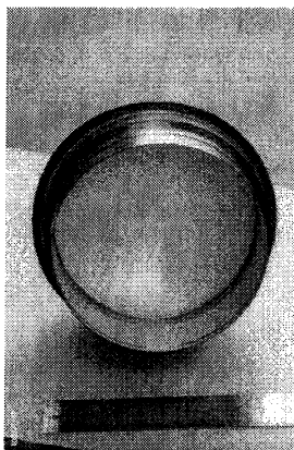
Fig. 8. Photo of CVD diamond disc before mounting in gyrotron ( a ) and after its failure ( b ).
