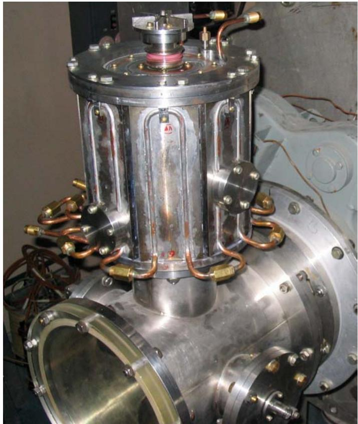
*Fig. 2. Photograph of the plasma driver on measuring vacuum chamber.*
