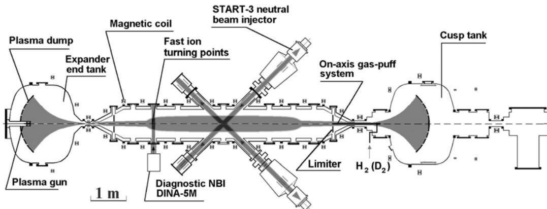
FIG. 1. Experimental model of gas-dynamic trap.
