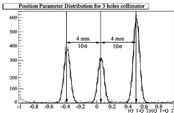
Fig. 7: Results of space resolution test of silicon PSD detector with alpha particles and three-hole collimator.
