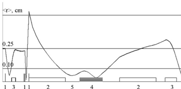
Fig 6: RMS beam size in AMS tract (calculations for  $W_0 = 15$  keV – initial energy,  $U_T = 1$  MV – terminal voltage), 1 – electrostatic lens, 2 – accelerating tube, 3 – double-focusing magnet, 4 –  $180^\circ$  combined bend, 5 – place of magnesium stripper.
