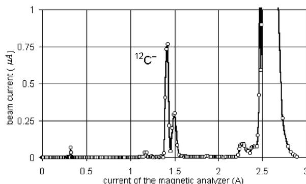
Fig. 5: Typical mass-spectrogram of negative ion beam from gas ion source (on  $\text{CO}_2$  gas).
