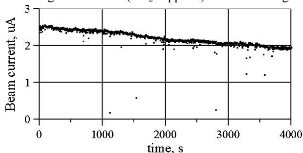
Fig. 4: Time dependence of  $\text{C}^-$  current from gas source in experiment.
