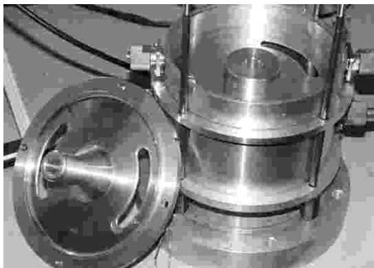
Figure 8: Accelerating structure (1:5 scale model).
