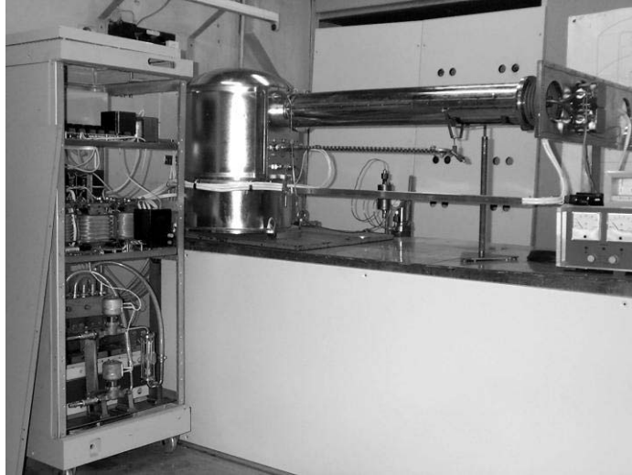
Figure 7. Liquid lithium rod – operating pre-prototype for final cooling .
