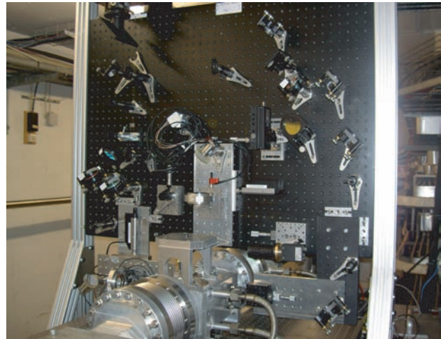
Figure 1. Picture of the laserwire breadboard installed at the PETRA positron storage ring.
