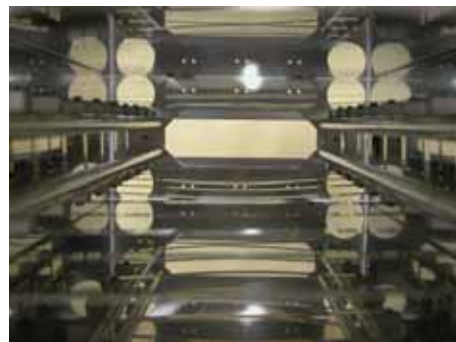
(b) View of inner conductor from the beam entrance
