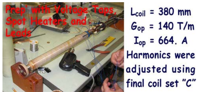
Figure 5. Completed QT Prototype Being Prepared for Vertical Cold Testing. During production we learned to decrease turn spacing and bend radius for a 7% transfer function gain.
