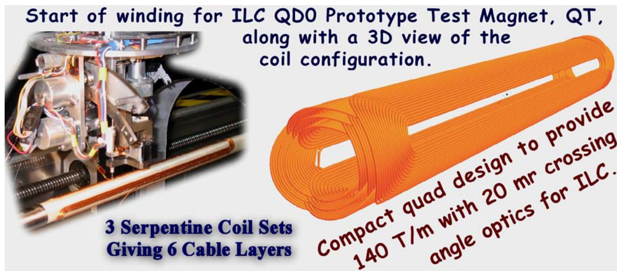
Figure 3. Winding the Short QD0 Magnetic Test Prototype, QT, and CAD Model of Final Six Layer Quadrupole Coil Pattern. QT production is complete along with warm field harmonic measurements. Quench testing was performed in an existing BNL dewar at 4.3 to 3.0° K temperature, 1 to 10 A/s ramp rates and solenoidal background fields up to 6 T. design requirements of 20 mm clear full aperture and 140 T/m operating gradient in the presence of a 3 T solenoidal background field. Figure 3 shows the start of QT coil winding along with full final coil structure. QT was produced in three winding steps as Serpentine style dual-layer coil sets A, B and C, for a total of six cable layers[8]. Before winding was complete warm magnetic measurements were performed and the results were used to make minor pattern corrections to the final coil set C.
