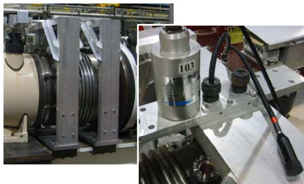
Fig. 9 Set up for the measurement of the vertical motion of the RHIC quadrupole cold mass.
