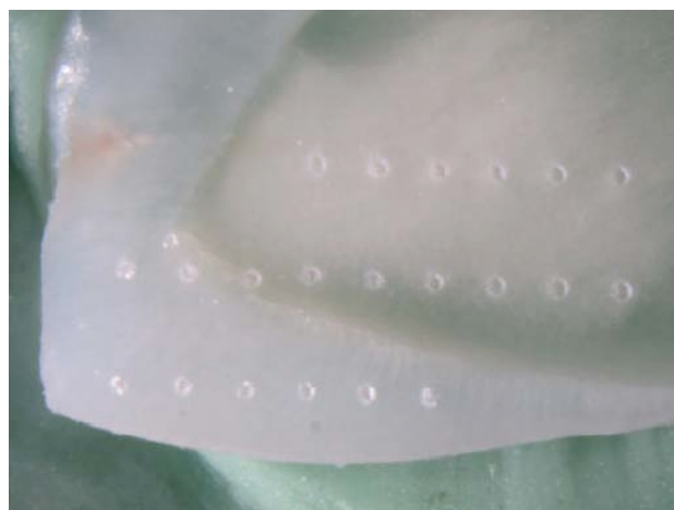
Figure 10: Holes on a human tooth drilled by ultrashort IR FEL beam of 2.94 \mu m [6].
