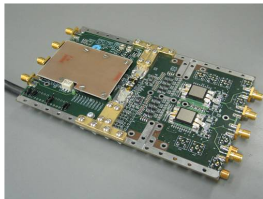
Figure 2: FONT3 solid-state amplifier with integrated feedback
