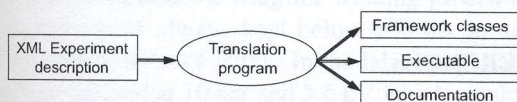
Figure 1: The translation program generates all codes of the framework from an experiment description. The framework is also linked and documented.
