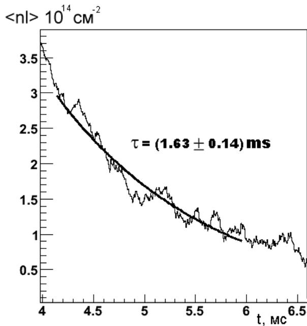
measured after plasma source was switched off. Radial profile of plasma potential is «stepwise».
