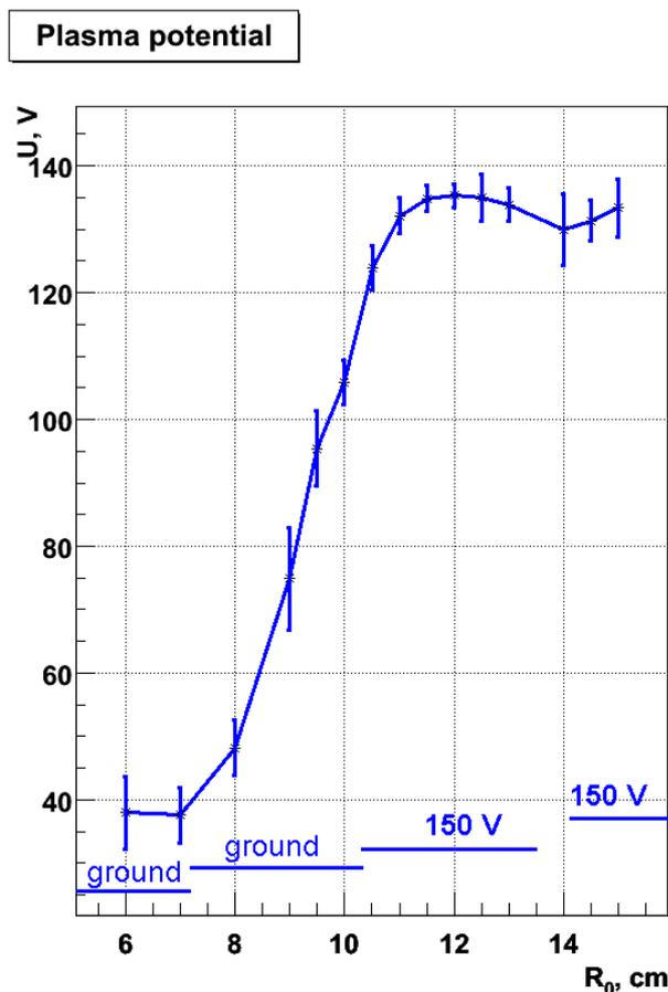
Fig. 2 Radial profile of floating potential in the central plane of GDT.
