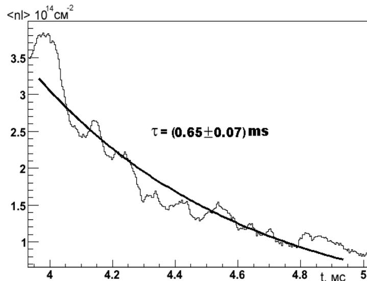
**Fig.4** Time evolution of electron linear density measured after plasma source was switched off. Limiters and plasma dump electrodes are grounded.
