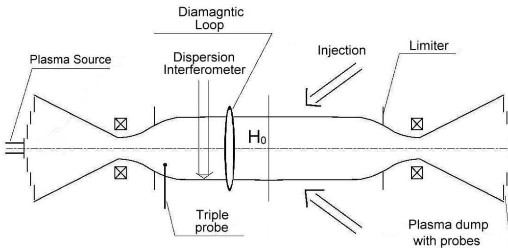
**Fig.1** Schematic view of the GDT magnetic field configuration, location of limiters, plasma dumps, diagnostics, plasma source and neutral beams.
