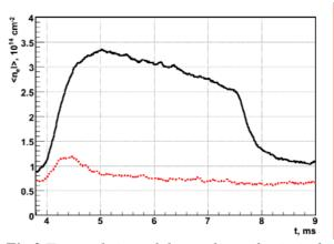
Fig.3 Time evolutions of electron linear density in the SHIP cell during Neutral Beam Injection (solid black line) and without injection (red doted line).
