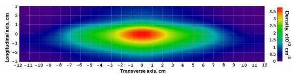
Fig.4 Spatial profile of SHIP fast ion density
