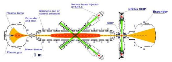
Fig. 1. SHIP experiment at the GDT device.
