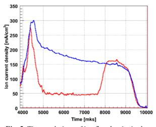
Fig. 5. Time evolutions of ion flux density in the expander cell with NBI in the SHIP cell (red) and without NBI (blue).
