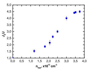
Fig.6 Ion flux suppression vs fast ion density.
