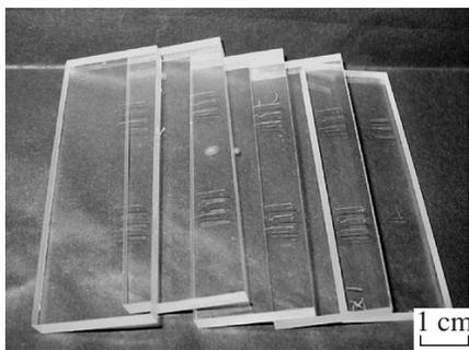
**Fig. 5.** Samples of polymeric MNFSs fabricated using a finished mask.
