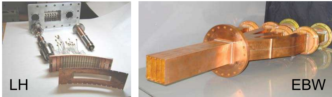
Figure 2: LH and EBW antennas shown before RF injection experiments.
