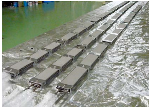
Figure 3: Three-layered NEG strip pump for antechamber.
