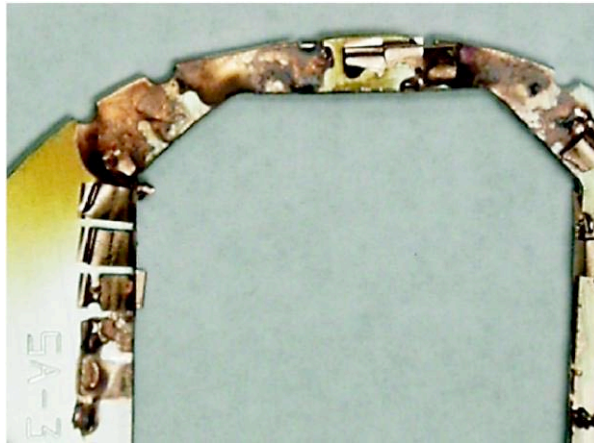
Figure 13: Damaged rf seal from a flex-flange connection.
