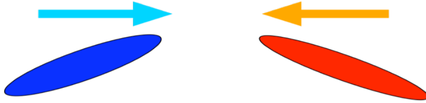
Figure 2: Collision with crossing angle is equivalent to head-on collision with tilt beam.
