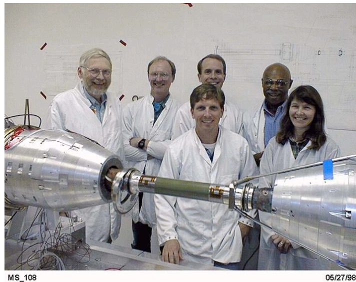
Figure 7: IR double-walled Be collision chamber with nearby water cooling and permanent magnet dipoles.
