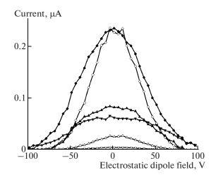
**Fig. 5.** Variation of the beam current at the exit from the AMS with electrostatic dipole voltage when quarter of the current is picked up from the body of the stripping target (empty circles) and when the beam is displaced in the transverse direction (filled circles). The target temperature characterizing the beam transmission is ( $\diamond$ ) 500, ( $\triangle$ ) 400, and ( $\nabla$ ) 350°C.
