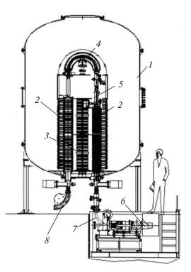
**Fig. 1.** Accelerator mass spectrometer: (1) tank for  $SF_6$ , (2) accelerating tube, (3) electrostatic filter, (5) magnesium vapor target, (6) ion source, and (7, 8) magnetic filters.
