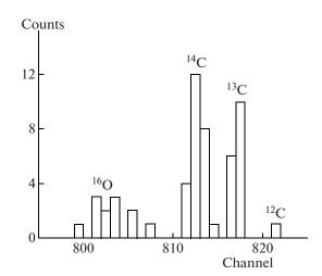
**Fig. 7.** Record of the  ${}^{14}$ C isotope present in the charcoal sample. The ordinate axis, number of events; the abscissa axis, the same as in Fig. 6.
