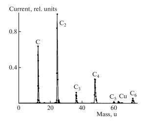
**Fig. 4.** Mass spectrum of negative ions produced in the sputtering ion source with the graphite sample.
