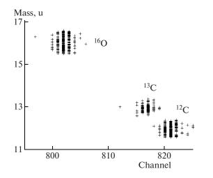
**Fig. 6.** Mass spectrum at the exit from the AMS under the conditions of scanning by the output magnet. On the abscissa axis, the time of flight of ions in the channels of the time-of-flight detector is plotted.
