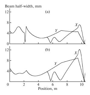
Fig. 2. Calculated transverse sizes of the beam along the AMS. The injection energy, accelerating voltage, and ion charge are (a) 30 keV, 2 MV, and 3+ and (b) 15 keV, 250 kV, and 1+.
