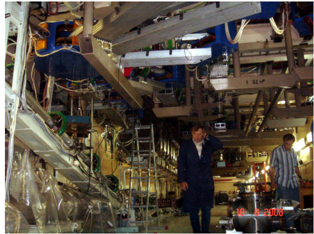
Figure 6: The bends are hung on the ceiling. Round magnet is at the top left corner, the old terahertz FEL magnetic system is at down-left. Elements of the optical resonator for the second-turn FEL are yet at the floor (down-right corner).
