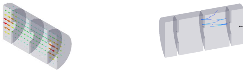
Figure 4: MultP-M: multipactor in DLW simulation results (left - electric field distribution, right – electron trajectory).
