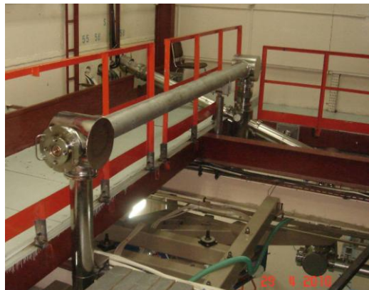
Figure 4: The optical beamline, which transports the radiation of the second FEL to the user stations.
