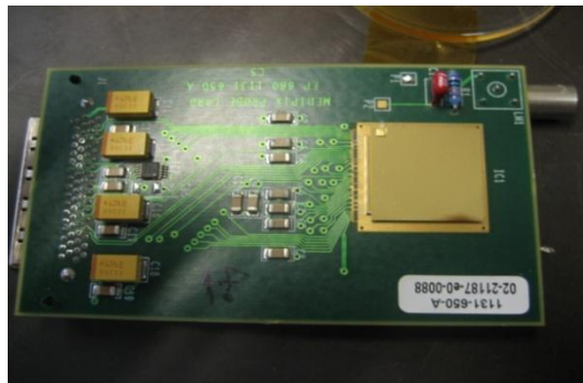
Figure 8: Spectrometric detector on basis of GaAs (Cr) pixel censor with 256 \times 256 channels of 50 \mu\text{m} resolution and Medpix chip.
