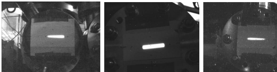
Figure 5: X-Ray beam from 7.5T SCW at output of three beam lines in the experimental hall of Siberia-2.
