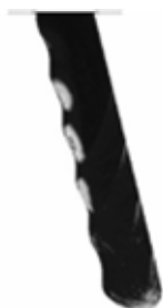
Fig.2: Capillary with wavy structure at the front; colour indicates absorbed intensity.
