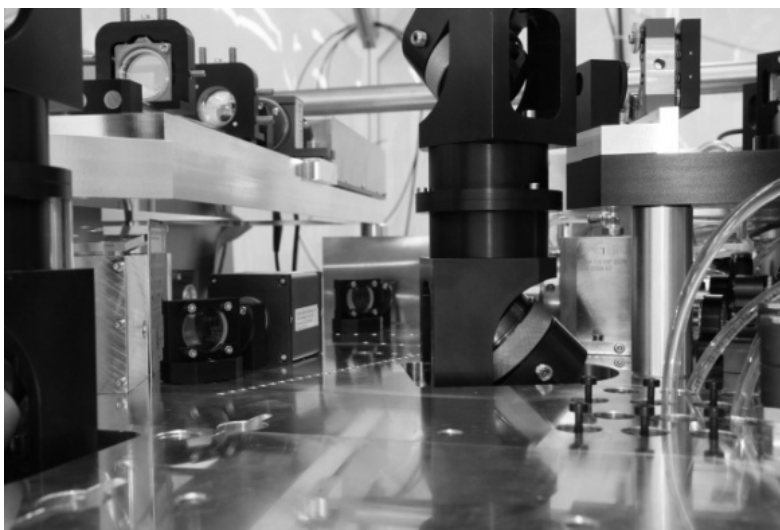
Fig. 1 View into 50 W laser VaryDisk offering pulse duration from 350 fs to 1 \mu s
