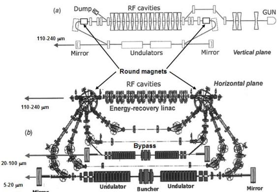
Other four orbits are in the horizontal plane. The beam is directed to these orbits by switching on of two round magnets. In this case electrons pass four times through acceleration RF cavities, obtaining 40-MeV energy. Then, (at the fourth orbit) the beam is used in FEL and decelerated four times.
