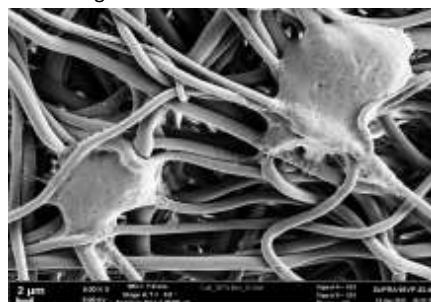
Fig. 1. Micrograph of a porous 3D matrix of chitosan containing 5 wt.% MMT
