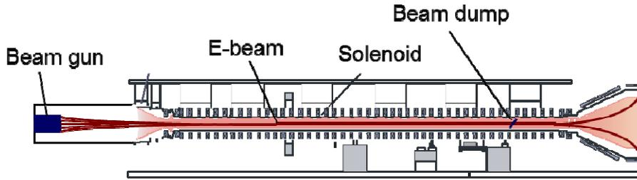
FIG.2. Layout of the GOL-3 experiment with 20 MW electron beam
