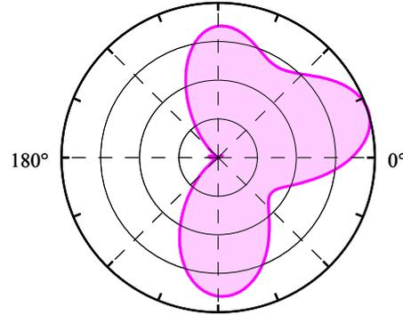
FIG. 4. Shape of reconstructed magnetic boundary in the disrupted shot PL11188 at  $t = 10 \mu\text{s}$ . Thick outer line corresponds to the limiter at  $a = 4 \text{ cm}$ . Distances between thin circles are of 1 cm.
