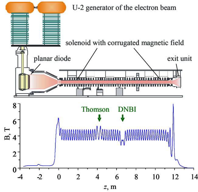
FIG. 1. Layout of the GOL-3 experiment (top) and axial dependence of the magnetic field (bottom). Axial coordinate  $z$  is measured from the centre of the high-field coil at the beam input side. Arrows at non-regularities of the magnetic structure indicate locations of Thomson scattering system and Diagnostic Neutral Beam Injector.
