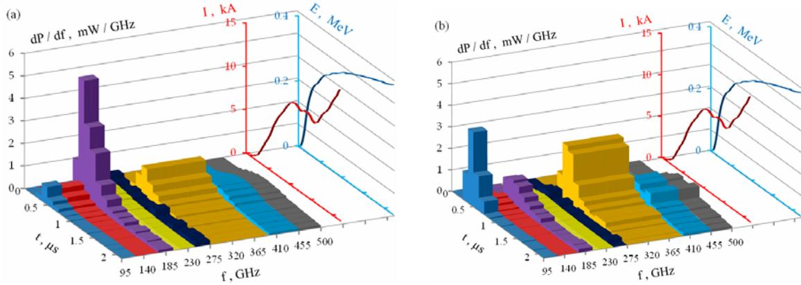
FIG. 7. Dynamics of the spectral power density of electromagnetic emission from the plasma with the polarization parallel (a), and perpendicular (b), to the magnetic field in the plasma.
