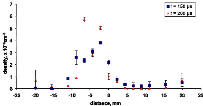
FIG. 8. Surface plasma density profile in PSI experiment measured by Thomson scattering. Two pulses laser beam (10 J, 30 ns, 1053 nm) passed at a distance of 9 mm from the surface of the W target.
