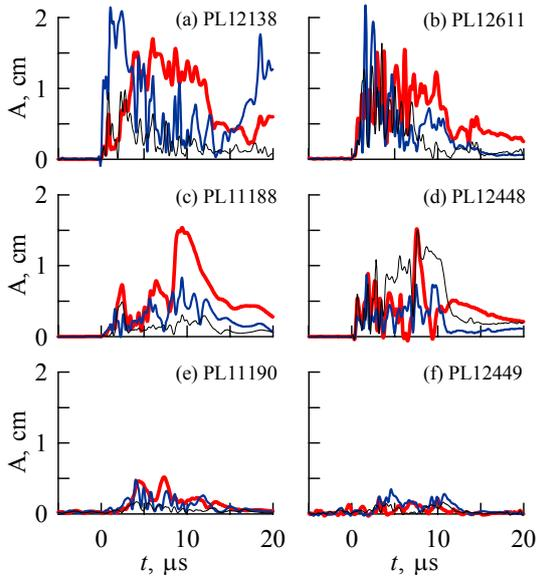
FIG. 3. Evolution of amplitudes of azimuthal modes  $m = 1$  (thick lines),  $m = 2$  (medium lines), and  $m = 3$  (thin lines) in shots with disruptions (a)–(d) and in normal shots (e), (f). The beam injection started at  $t = 0$ .
