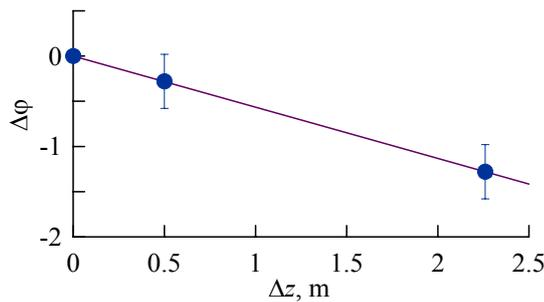
FIG. 5. Dependence of the phase on the coil distance relatively to the 16-channell array.
