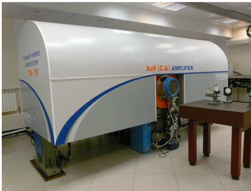
Figure1. Photo of the XeF(C-A) amplifier optically driven by e-beam-to-VUV-radiation converter (THL-100 femtosecond system, Tomsk, Russia).
