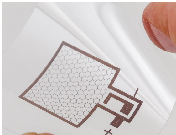
Figure 1. Laser printed silver paste based current spreading bus bar structures for OLED applications.
