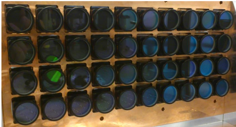
Figure 1. Mirror array of multi-pass amplifier to geometrically fold the beam path 40 times on the amplifying thin-disk crystal.
