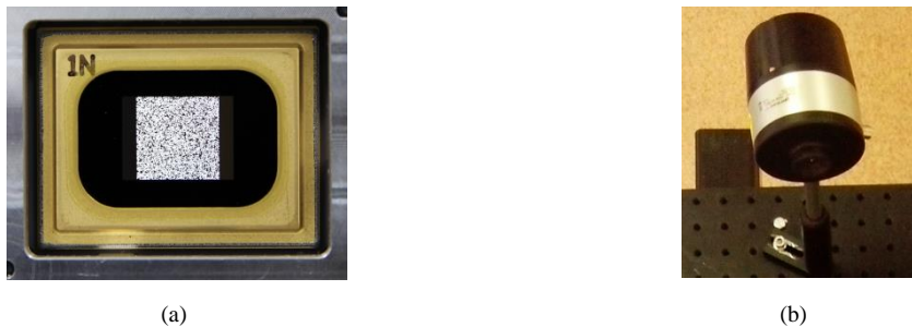
Figure 1. (a) DMD projecting one of the encoding masks of 63/65 pixels in bundle of 12/12 micro-mirrors. (b) Pyroelectric detector 0.1-30 THz range
