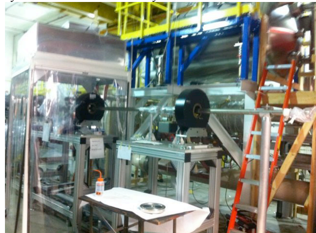
Figure 8: Assembling of the in the low-energy beam-line. Black round magnets are two of five solenoids in this section.
