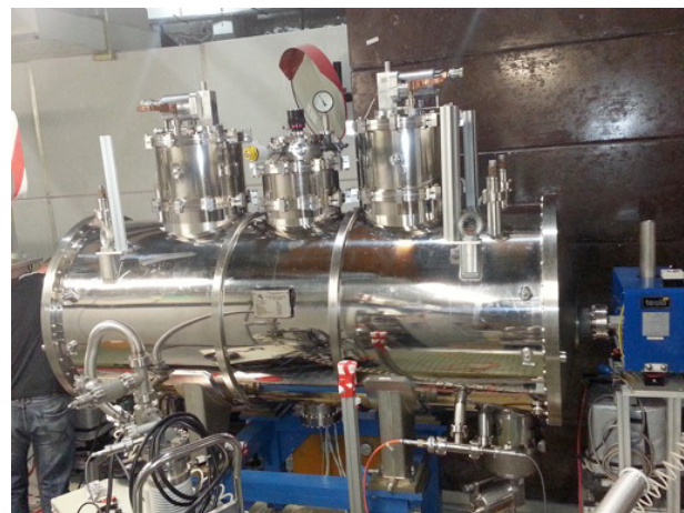
Figure 1: The refurbished superconducting wiggler installed in the Elettra storage ring.
