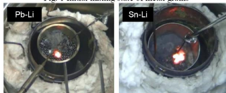
Fig. 2 Small fire generation during fabrication of alloy by melting and mixing
