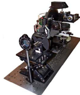
Fig. 8. ST-100 He flow cryostat and sample unit with precise focusing of pump and probe terahertz beams for study of transient absorption with 100-ps resolution.
