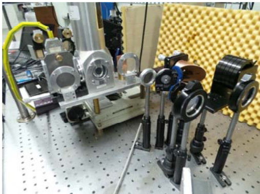
Fig. 8. ST-100 He flow cryostat and sample unit with precise focusing of pump and probe terahertz beams for study of transient absorption with 100-ps resolution.
