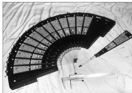
Fig. 7. The first fast one-coordinate scintillation X-ray detector for digital differential angiography on synchrotron radiation (spatial resolution: 1.5 mm, number of channels: 128, count rate: 128 \times 1 MHz).
