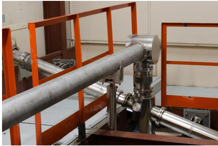
Figure 4: Optical beamline for FELs. Radiation of all FELs is delivered to the same user stations. Switching between FELs is done using retractable mirrors.
