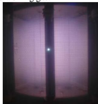
Fig 2. Picture of a single segment discharge experimental set up, with argon as working gas.
