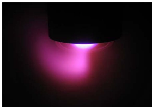
Fig.1. Side view photograph of the dual magnetron with closed magnetic field and tilted magnetrons.
