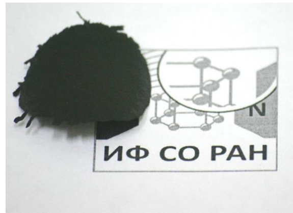
Fig. 1. A typical image of the film flexible absorber based on diamond-graphite mixture and polyethylene
