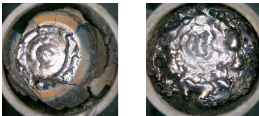
Fig. 1. The image of the surface formed as a result of laser irradiation of hafnium carbide (the left) and of Hf-C mechanocomposite (the right).
