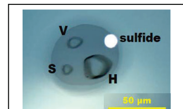
Figure 2: The image of a melt inclusion in olivine with volatile (V), hydrogen isotope (H), and sulfur isotope (S) measurement pits. (modified from [2])
