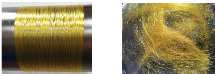
Figure 2. Polymer fibers of garnet composition
