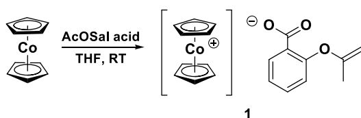
Scheme 1. Synthesis of cobaltocenium acetyl salicylate ( 1 ).
