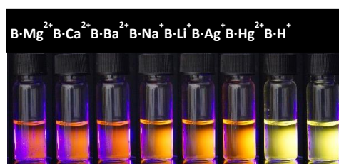
Figure 1. Fluorescence changes of bisstyryl (B) after addition of 10 equivalents of different metal ions.
