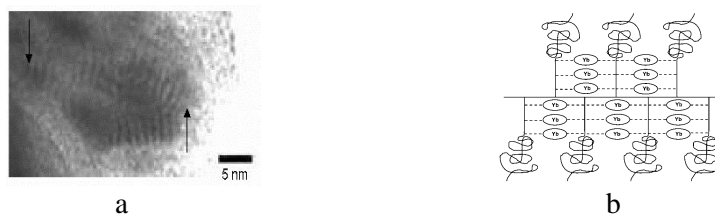
Fig. 1. (a) TEM micrograph and (b) schematic representation of the architecture of a conjugate between PI-g-PMAA molecular brush and Yb(III)-porphyrzine complex.
