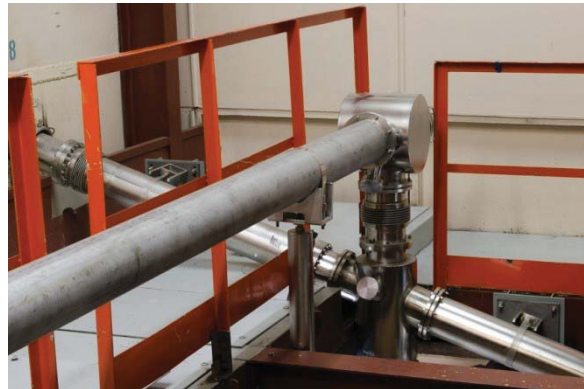
FIGURE 6. Optical beamline for FELs. Radiation of all FELs is delivered to the same user stations. Switching between FELs is done using retractable mirrors.
