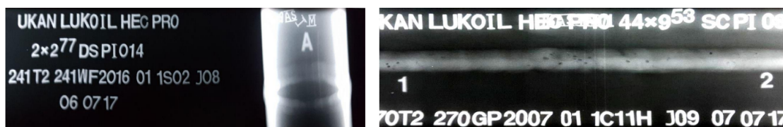
Figure 1: X-ray picture of welded seam sample (∅=50.8 mm) received by ionizing radiation source of Ir-192.
