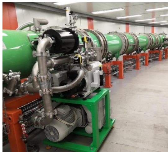
Figure 1: Booster ring inside Synchrophasotron yoke.
