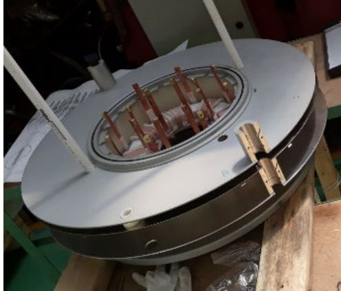
Figure 2: A photo of the prototype of the cascade transformer based on a distributed windings.
