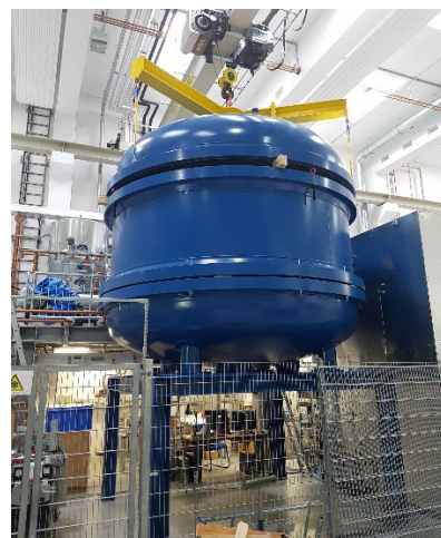
Figure 2: "Big-Blue-Bubble" HV tank with still open flanges.
