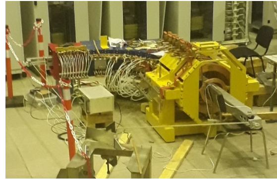
Figure 7: Part of cooler's transport channel during magnetic measurements. The assembling consists of 3 solenoids (called "INSERT" (red), "BEND" (blue) and "LINE-08" (yellow)). Aluminium rail of needed bent shape is installed inside the solenoids.
