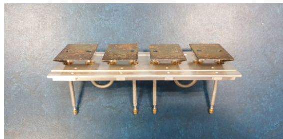
Figure 1: Set of four electrodes (length of support 175.4 mm) powered by a single amplifier (see text).
