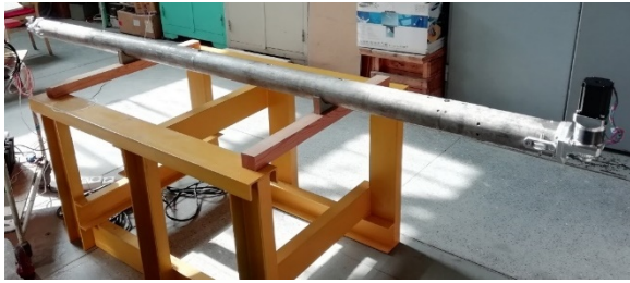
Figure 9: titanium rail for compass-based measurements
