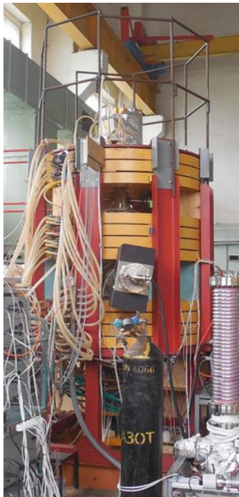
Figure 2: A photo of the test stand for the electron gun.
