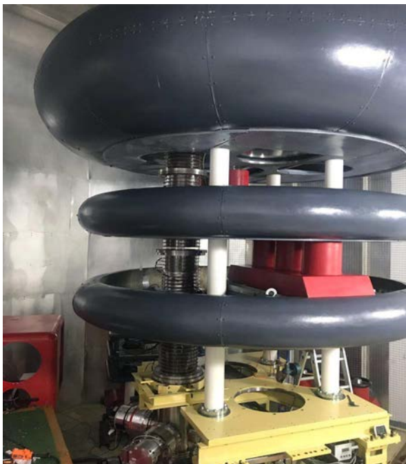
FIG. 18. Photograph of 0.72 MV Electrostatic Quadrupole (ESQ) accelerator completed (reprinted from Fig. 1 of Ref. [146] Copyright (2020) with permission from Elsevier).
