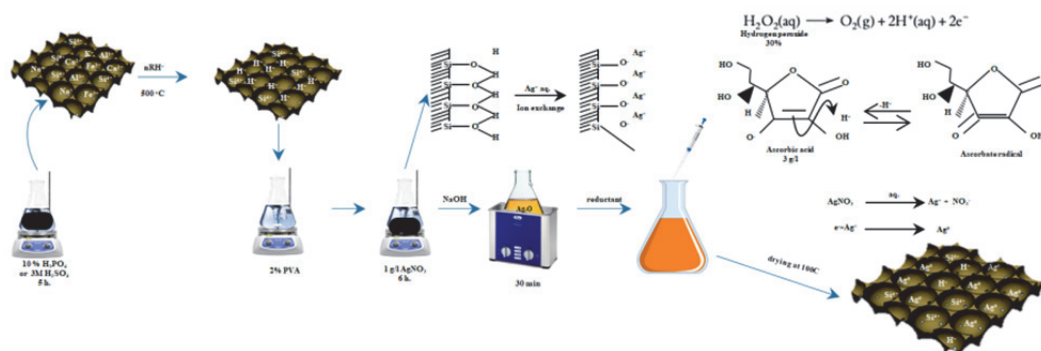
Stages of synthesis of silver nanoparticles on the surface of diatomite and kaolin
