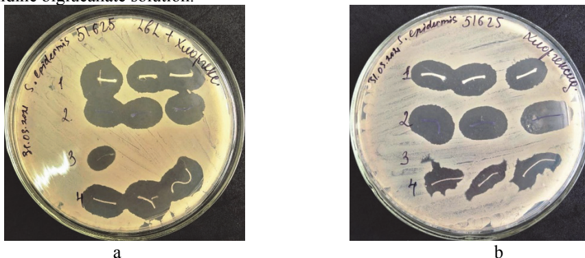
Results of the antimicrobial activity of surgical threads against Staphylococcus epidermidis ATCC 51625: 1 – rumasan, 2 – rumacryl, 3 – polypropylene, 4 – Polyamide; a - surgical threads treated with CMC-Na-chitosan and chlorhexidine biglucanate solution, b - surgical threads treated with chlorhexidine biglucanate solution
